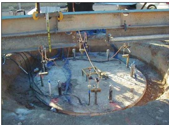
**Figure 5.** Bi-directional test in progress (at 163 MN) West Virginia, USA
