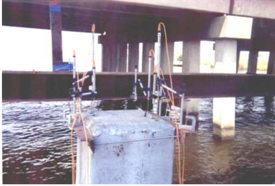
**Figure 14** Testing of pre-cast pile over water.
