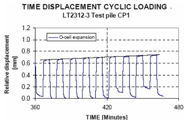
**Figure 11** –Displacement Time Chart for 100 minute cyclic loading
