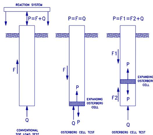
**Figure 6.** Test method comparison
