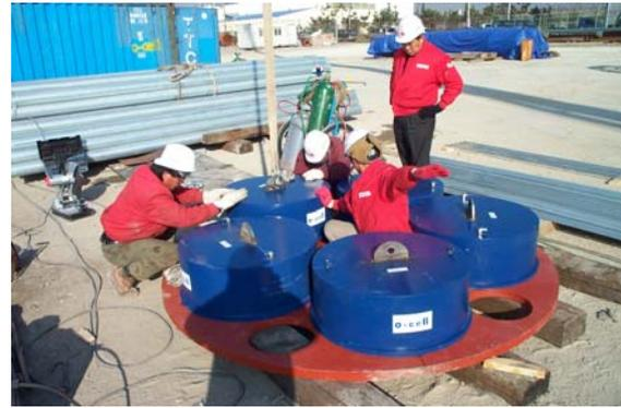
**Figure 3** Multiple O-cell assembly for a 3m diameter pile in Korea.
