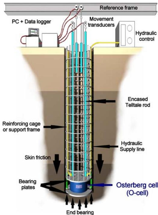
Figure 7. Bi-directional test schematic
