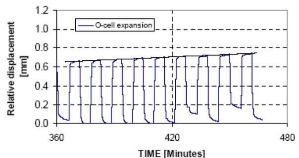
**Figure 11** –Displacement Time Chart for 100 minute cyclic loading
