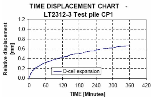
**Figure 9** –Displacement Time Chart for 6 hour hold of constant load
