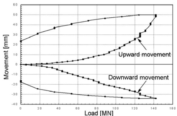
Figure 8. Load-Movement Curves Incheon Bridge - Korea
