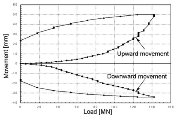
Figure 8. Load-Movement Curves Incheon Bridge - Korea
