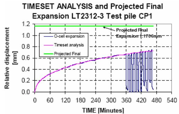
**Figure 10** –Displacement Time Chart showing cyclic loading and additional displacement
